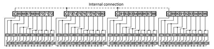
**Note:** For connecting the load of the double electro-valves on the *expansions* (ECOMATIC-S 64/96) it is necessary to do one *connection* between the terminal C (common) of the expansion board and the terminal C of the ECOMATIC-S32 board.
