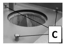
Side doors to clean air and row air chambers are dismounted. All filter bolts in clean air chamber are screwed completely down (point C).
