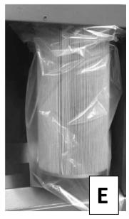
Bolts for filter cones are removed (point D). Now the filter cartridges can be removed.
