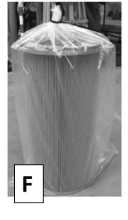
The new filter cartridges (check sealing) are hung on the filter bolts. They are fastened hereafter (point G). Doors are mounted.
