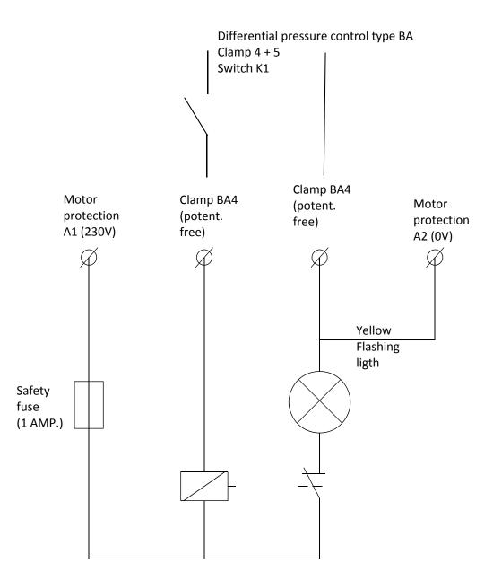
Power from motor protection (A1 and A2) may only be supplied, when fan is in operation with 230VAC and 0VAC.
