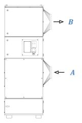
Process air is led in at (A), where after the air passes the pre-separator and filter elements.
