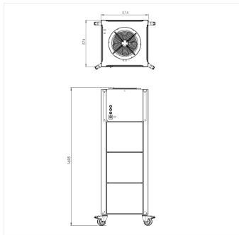
The E-PURE ASPRA M2500 is a mobile filter, specifically designed for usage in large rooms.
