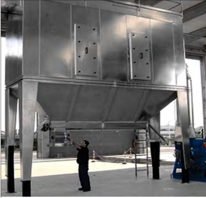
BFEMP with endless screw and rotary valve
