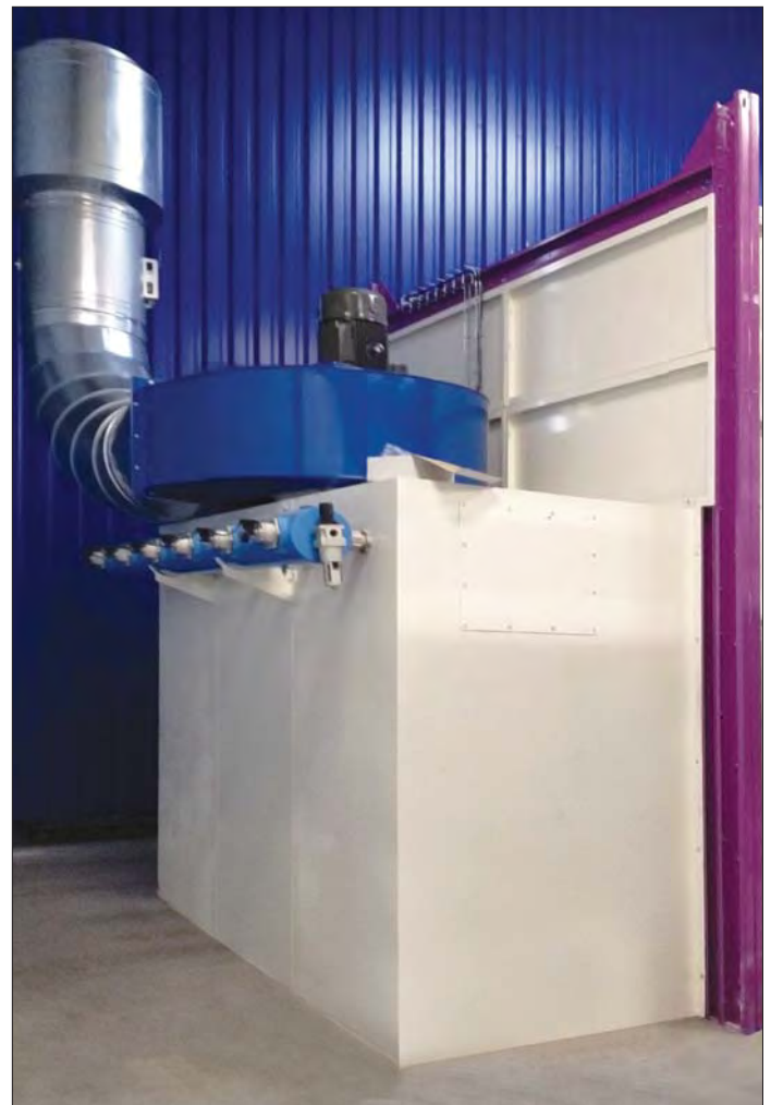
Suction wall with fan mounted, fully integrated in paint booth
