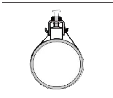
Reed contact supplied with strap to fix to cylinder
